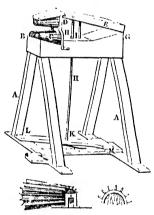
the upper conical roller, is attached to the main frame by a moveable joint at its upper end, and is connected near its other
